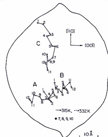
FIG. 3. A map for the three Re atoms shown in Fig. 4. Atoms A and B migrated together until B fell into a potential trap. B started to move again only when the heating temperature was raised to 332 K.
