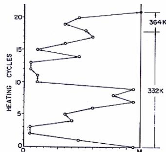
FIG. 1. One-dimensional discrete random walks of a Re atom on a W (123) plane. The diffusion is along a surface channel. Each jumping step is 2.74 Å, and the channel has a total of 17 steps.
