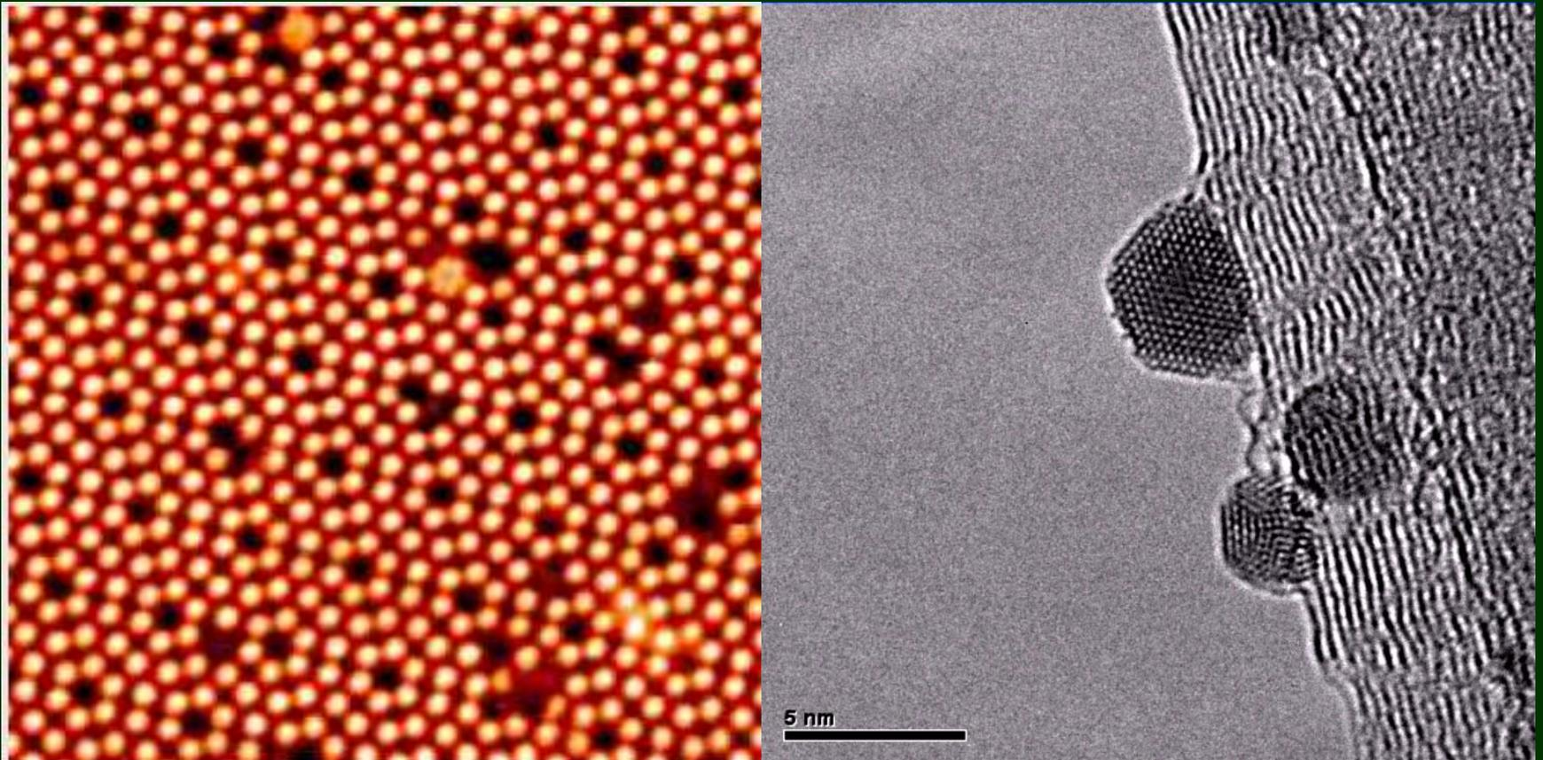
**STM & TEM Images of Si(111)-7x7 Surface & Ag Nano Crystals Grown on Multiwall Carbon Nanotube**
