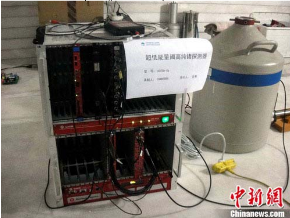
A germanium detector made by germanium crystal material with the highest purity in the world. (Photo by Chinanews.com)
