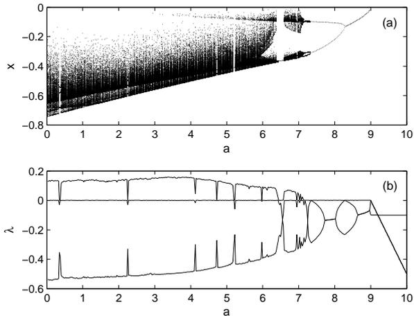
FIG. 1: (a) Bifurcation diagram based on the Poincaré section ( $z = 0$ ); (b) Lyapunov exponents spectra ( $\lambda_1 \geq \lambda_2 \geq \lambda_3$ ).
