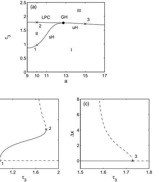
FIG. 7: (a) Bifurcation curves in parameter space  $(a, \tau_3)$ ; Branches of limit cycles and the steady state: (b) for the fixed value  $a = 10$  and (c) for  $a = 15$ .
