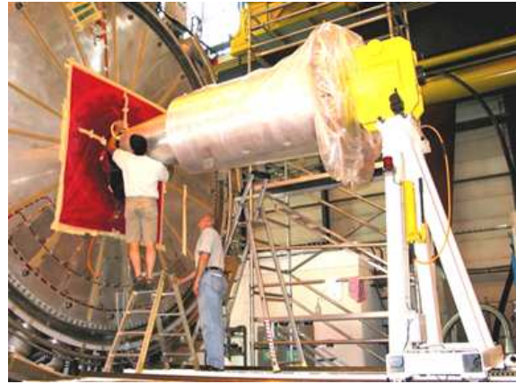
Figure 5.24: Completed FCal assembly with its bulkhead and cone attached, just before insertion into the end-cap cryostat.
