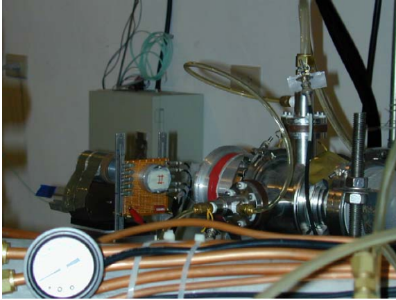
Fig. 2. Faraday cup and irradiation window in the external proton beam line.
