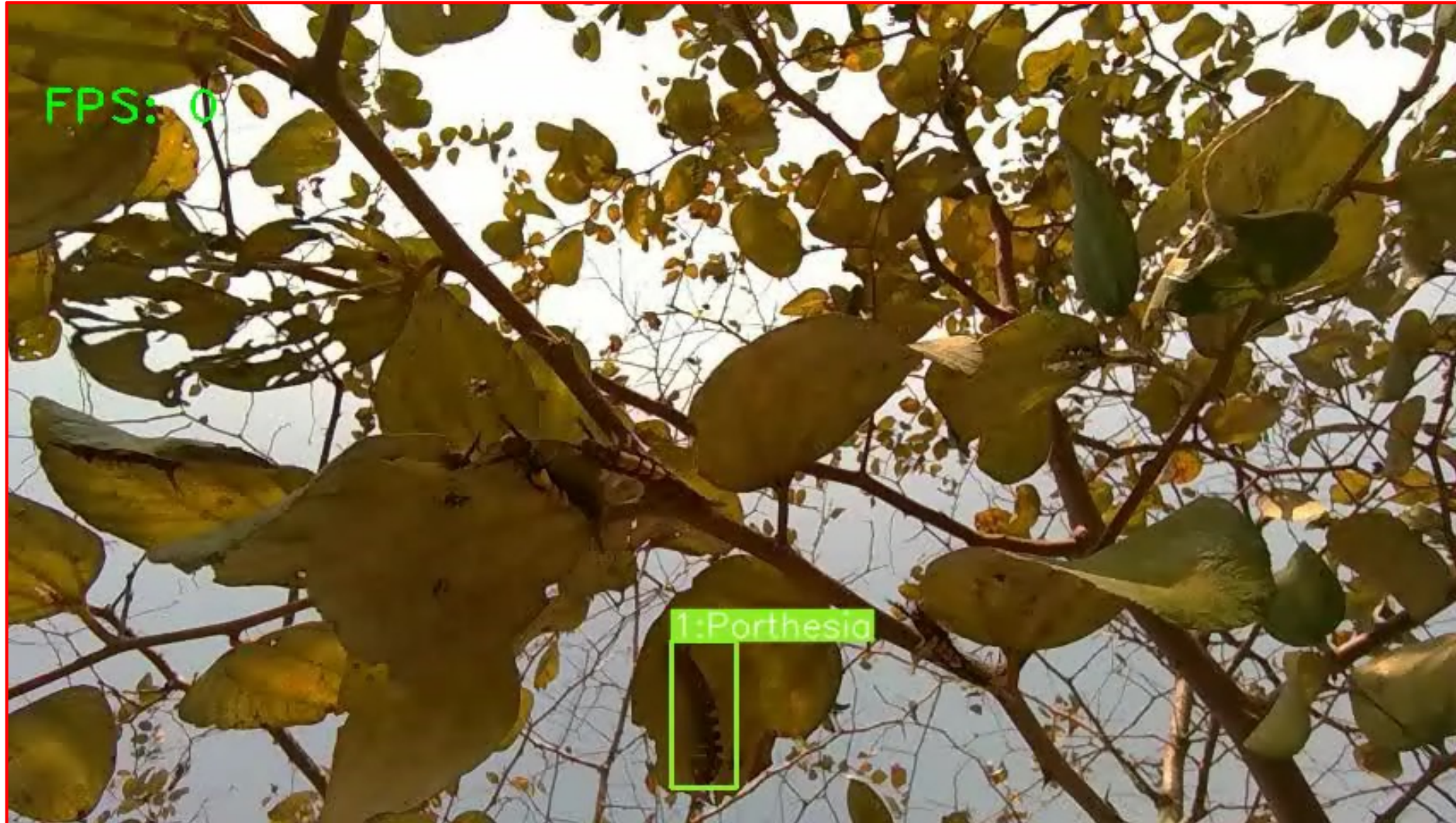
Detection and tracking at 15-20 cm (YOLOv7+SORT)
