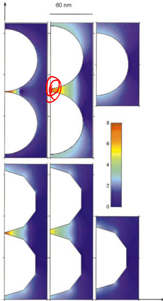
FIG. 3. (Color) EM-enhancement factor M^{EM} at a cross section through six different silver particle configurations. The wavelength of the incident field is \lambda = 514.5 nm with vertical polarization. The left-hand column illustrates the EM enhancement for dimer configurations of two spheres (top) and two polygons (bottom) with a separation of 1 nm. The middle column shows the same situation, but with a separation distance of 5.5 nm. The right-hand column shows the case of an isolated single particle. All particles share a common largest dimension of 90 nm. Note that the color scale from dark blue to dark red is logarithmic, covering the interval 10^0 < M^{EM} < 10^8 . Regions with enhancement outside this interval are shown in dark blue and dark red, respectively.
