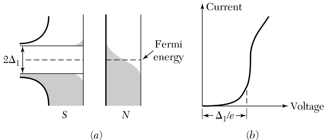
The density of states and the current-voltage characteristic for a tunneling junction.
