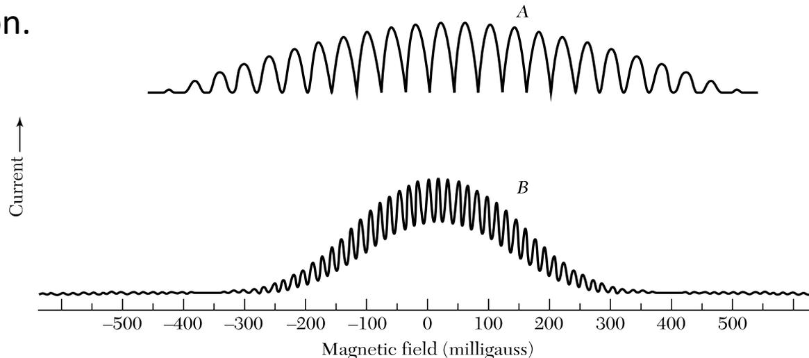
The field periodicity is 39.5 and 16 mG for *A* and *B*, respectively. Approximate maximum currents are 1 mA (*A*) and 0.5 mA (*B*). The junction separation is 3 mm and junction width 0.5 mm for both cases. The zero offset of *A* is due to a background magnetic field.
