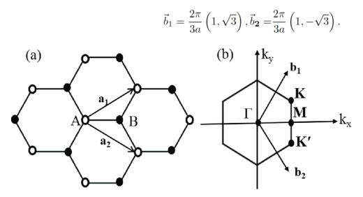
(a) Honeycomb lattice structure of graphene. The unit cell consists of carbon atoms represented by A and B,  $a_1$  and  $a_2$  are the lattice vectors and (b) corresponding Brillouin zone of graphene at origin ( $\Gamma$ ) with two Dirac points K and K' with the reciprocal lattice vectors
