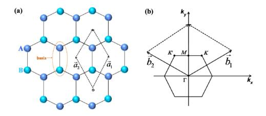
(a) The honeycomb crystal structure of graphene. The unit cell, rhombus, defined by vectors  $\vec{a}$  and  $\vec{a}$  a2 containing two atoms belonging to sublattices A (blue) and B (cyan) are highlighted in light blue. (b) shows the graphene Brillouin zone in momentum space. The points K and K ' denote the position of Dirac points while  $\vec{b}$  b1 and and  $\vec{b}$  2 represent the reciprocal lattice vectors
