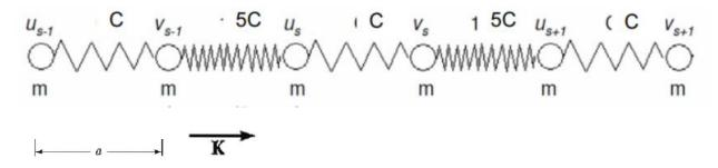
Each site has bond with force constant C on one side and 5C on the other side.
