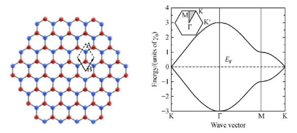
Honeycomb lattice structure of graphene consisting of two atoms (A and B) and Phonon spectra of graphene. The low energy band structure exhibits zero energy gap at the Dirac point.
