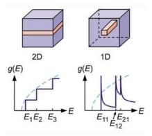
Electronic density of states g(E) in isotropic semiconductors (red), clad by barriers (blue) in 2D quantum well and 1D quantum wire. The dashed curve represents the 3D case drawn for reference.
