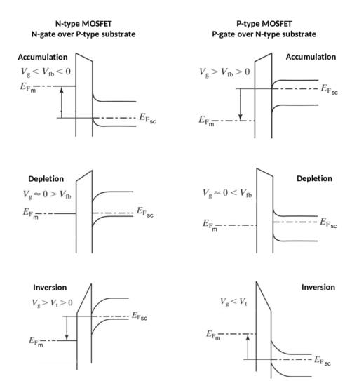
1. **Carrier Accumulation:** In accumulation, there is a buildup of majority carriers (electrons for n-type, holes for p-type) at the interface due to an applied voltage. The energy band diagram shows a flat band condition near the interface. The charge distribution reveals an excess of electrons (for n-type) or holes (for p-type) at the surface.
