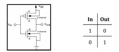
Input High (Logic 1): When a logic high input voltage is given to the CMOS inverter, the PMOS (p-type) is switched OFF, providing a high-resistance path to VDD whereas the NMOS (n-type) is switched ON, creating a low-resistance path to ground. Thus, the output is pulled down to ground, resulting in a low logic output voltage.
