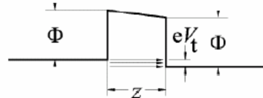
FIG. 3. Energy diagram of an idealized tunneling gap. The image charge effect (see Chen, 1993) is not taken into account here.
