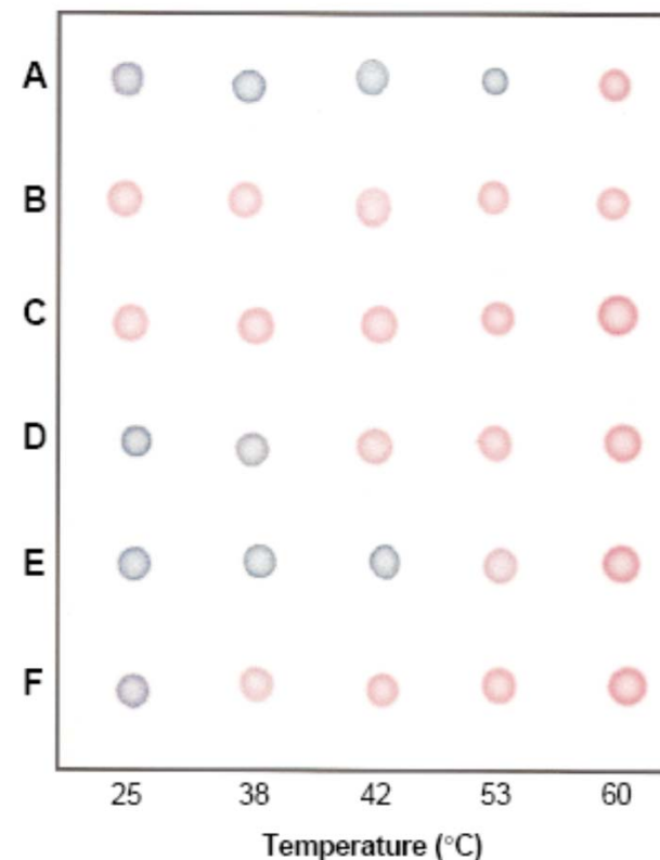
Fig. 4. Selective polynucleotide detection for the target probes shown in Fig. 2: (A) complementary target; (B) no target; (C) complementary to one probe; (D) a 6-bp deletion; (E) a 1-bp mismatch; and (F) a 2-bp mismatch. Nanoparticle aggregates were prepared in a 600- \mu l thin-walled Eppendorf tube by addition of 1 \mu l of a 6.6 \mu M oligonucleotide target to a mixture containing 50 \mu l of each probe (0.06 \mu M final target concentration). The mixture was frozen (5 min) in a bath of dry ice and isopropyl alcohol and allowed to warm to room temperature. Samples were then transferred to a temperature-controlled water bath, and 3- \mu l aliquots were removed at the indicated temperatures and spotted on a C 18 reverse phase plate.
