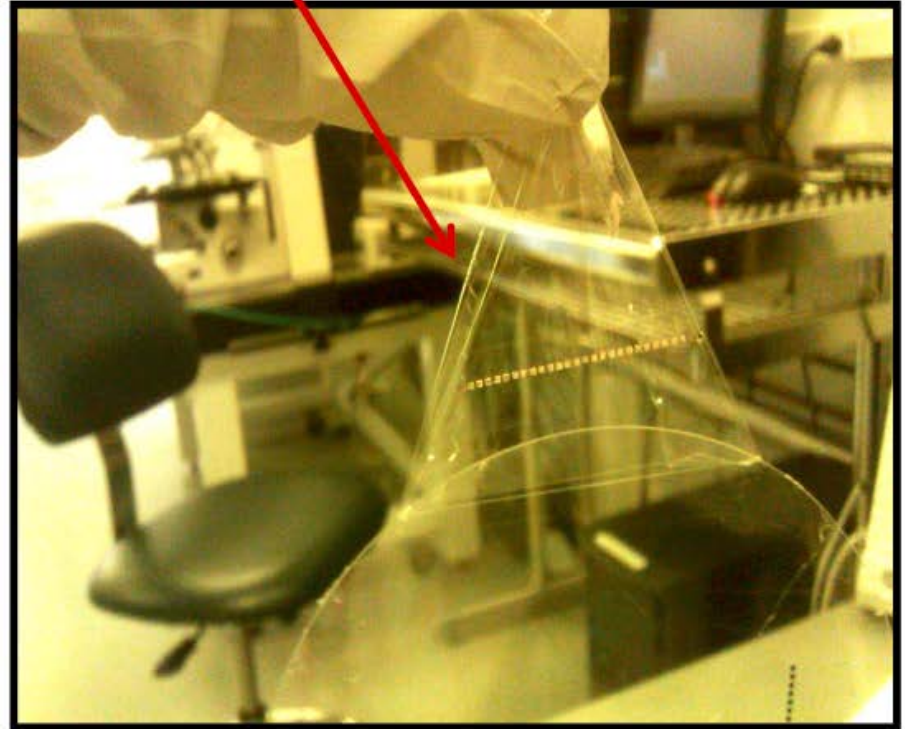
Parylene C – 4 \mu\text{m} thick
