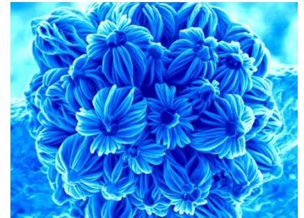
A 3-dimensional nanostructure grown by controlled nucleation of Silicon-carbide nanowires on Gallium catalyst particles
