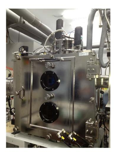
• Application: Deposition of metallic layers (Cu, Zn, Sn), and metal oxide layers(ITO, ZnO).
