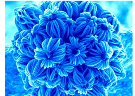
A 3-dimensional nanostructure grown by controlled nucleation of Silicon-carbide nanowires on Gallium catalyst particles – Univ. of Cambridge, 2007
