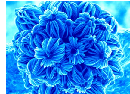
A 3-dimensional nanostructure grown by controlled nucleation of Silicon-carbide nanowires on Gallium catalyst particles
