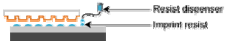
Step 2: Dispense drops of liquid imprint resist
