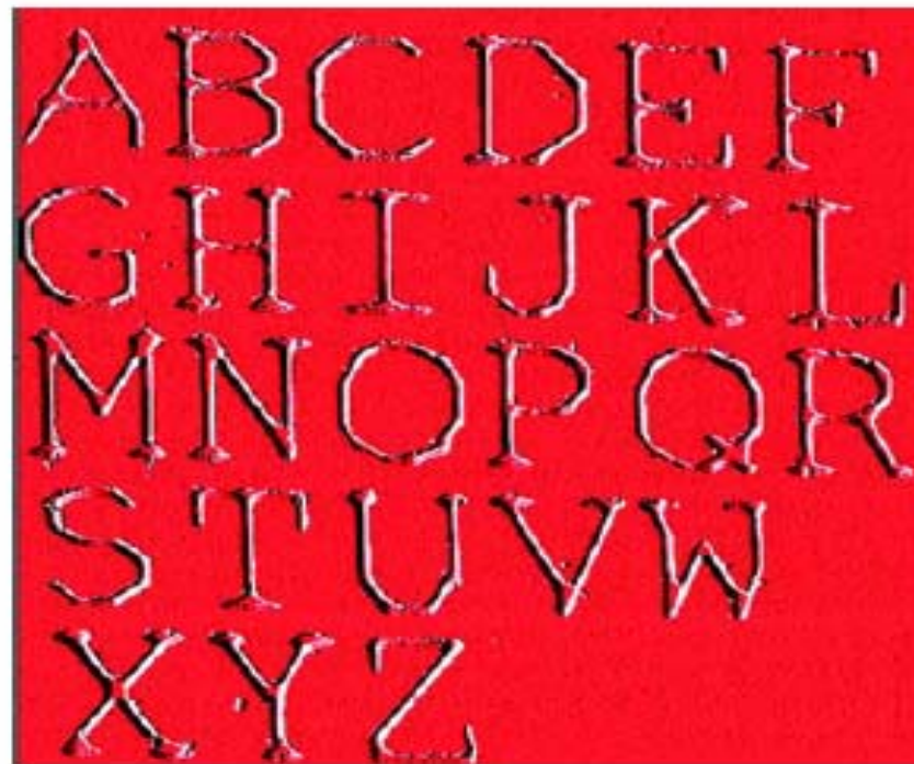
Figure 2. TappingMode image of a lithography test pattern. The Aurora-3 used nanolithography software to write into S1805 photoresist. 25 \mu m scan.
