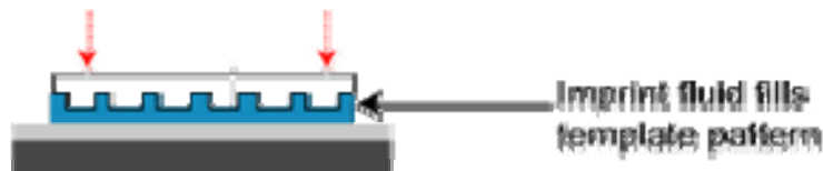
Step 3: Lower template and fill pattern
