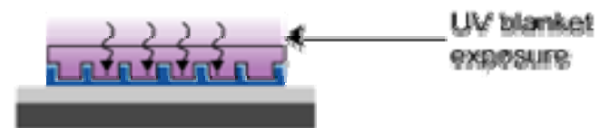
Step 4: Polymerize imprint fluid with UV exposure
