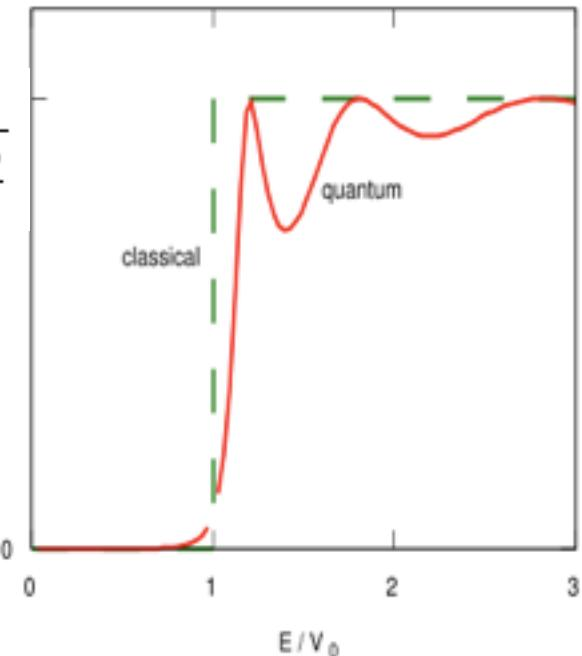
Transmission probability of a finite potential barrier for
