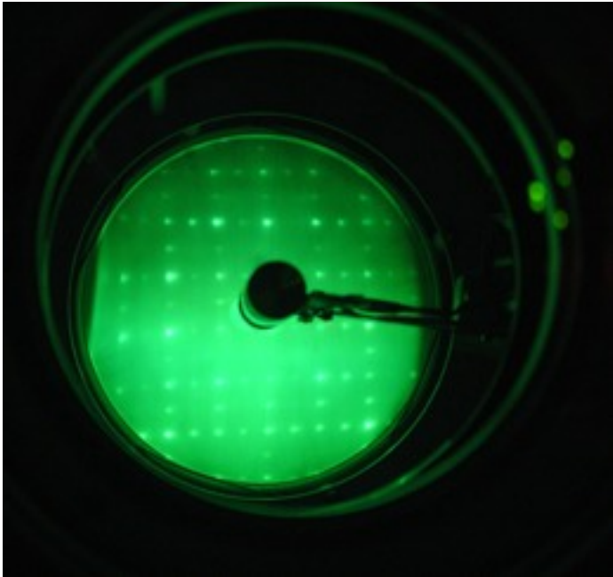
LEED pattern acquired on Si(100) surface
