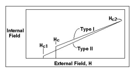
Type I superconductors are comprised of pure metals, whereas Type II superconductors are comprised primarily of alloys or intermetallic compounds.
