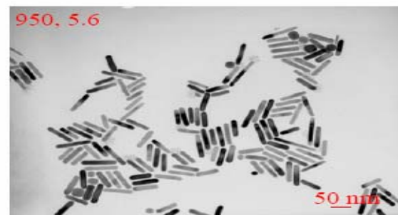
Figure 1-6: The absorption spectra of gold rods of different aspect ratios (left) and TEM of the rods with aspect ratios at 2.4, 3.9 and 5.6.
