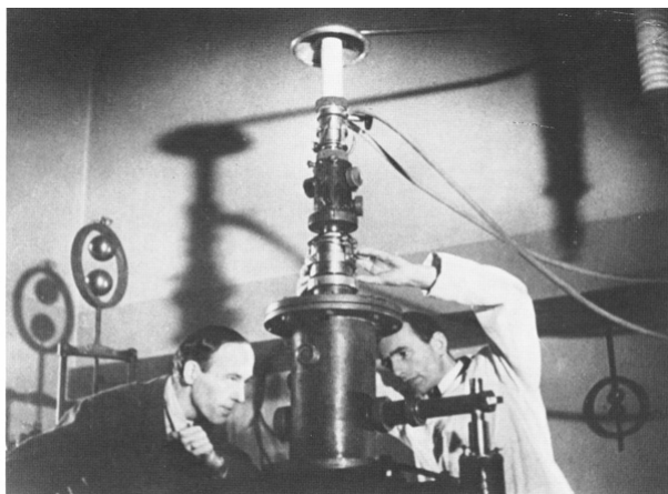
Fig. 6. The first electron microscope. The publication (48) contained only one cross-sectional drawing corresponding to Figure 5. This photograph, reproduced here for the first time, with M. Knoll and the author – was actually taken several years later, on 8 February 1944.
