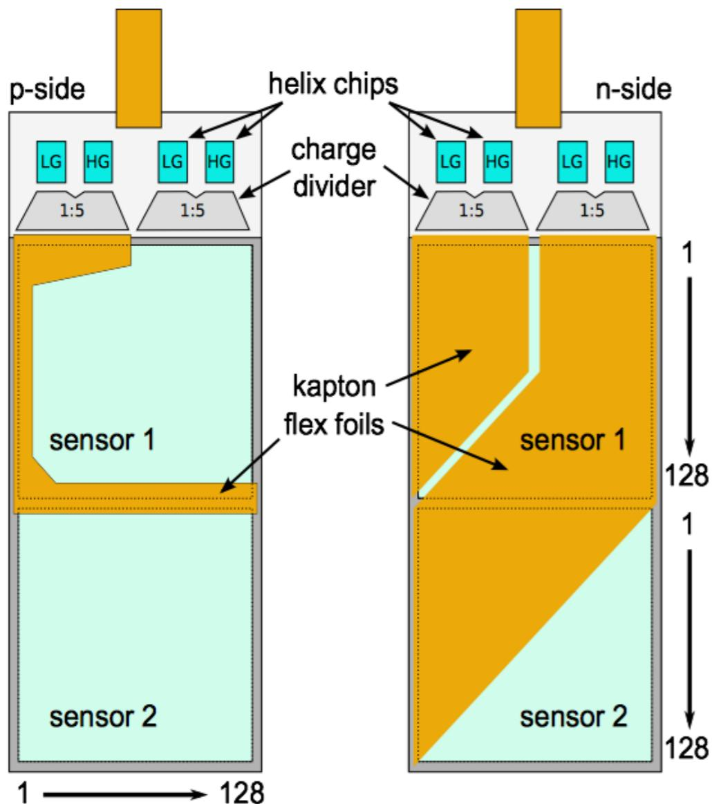
Schematic design of the scintillating fibre tracker (SFT)
