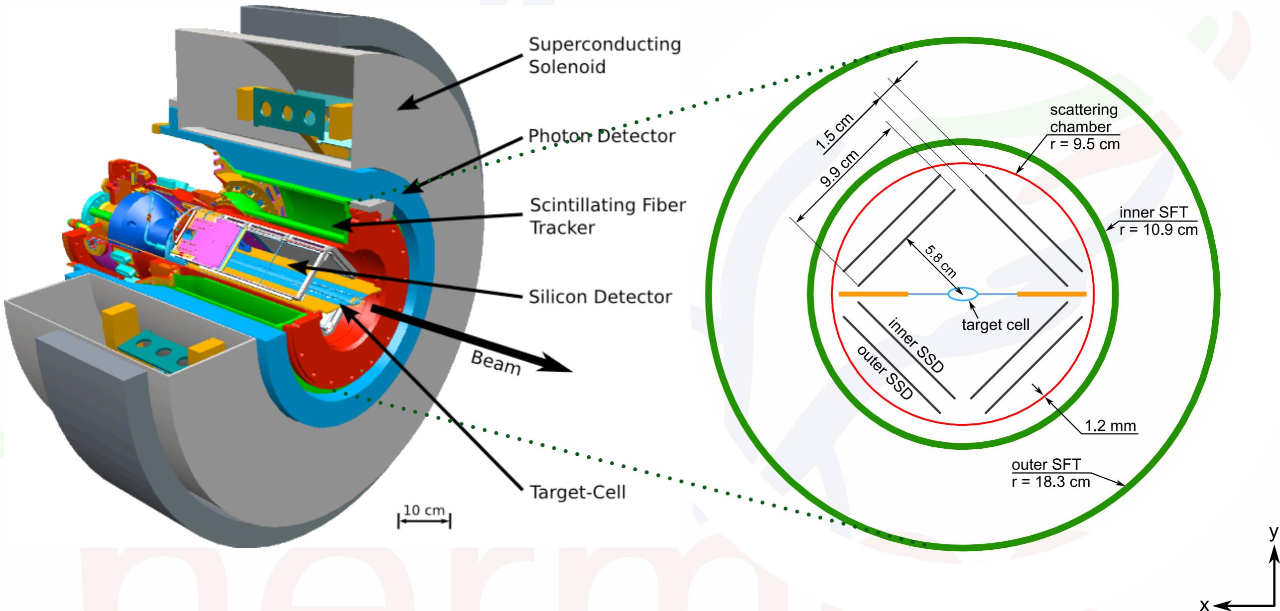
Enables the measurement of the recoiling charged particle and therefore full  $e p \rightarrow e p \gamma$  event reconstruction
