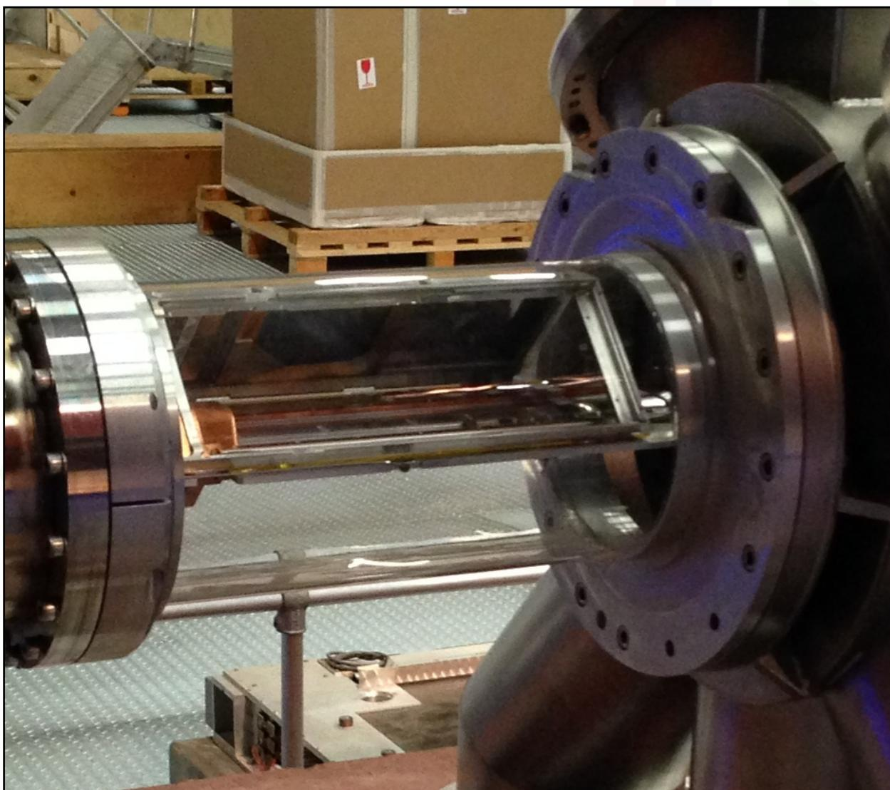
The scintillating fibre tracker (SFT)
