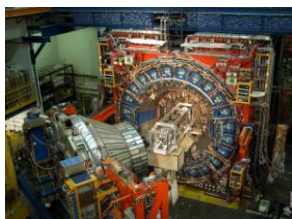
1: Insertion of the silicon track into the CDF II detector.
