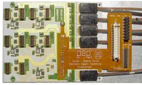
2: Silicon tracker read out Port Card mounted with the “Dense Optical Interface Modules” (black chips with optical fibers)
