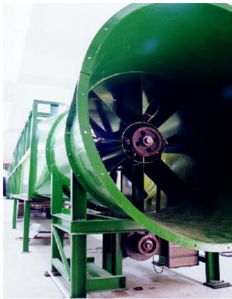
Fig. 1. View of the Environmental Wind Tunnel (Total length 22.6 m, and test section: 12.6m (L) x 2 m (W) x 1.4~1.6 m (H); speed range 0~20 m/s; Motor power of the 10-blade axial fan: 75 HP)
