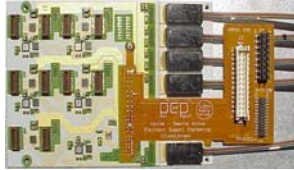
2: Silicon tracker read out Port Card mounted with the "Dense Optical Interface Modules" (black chips with optical filbers)
