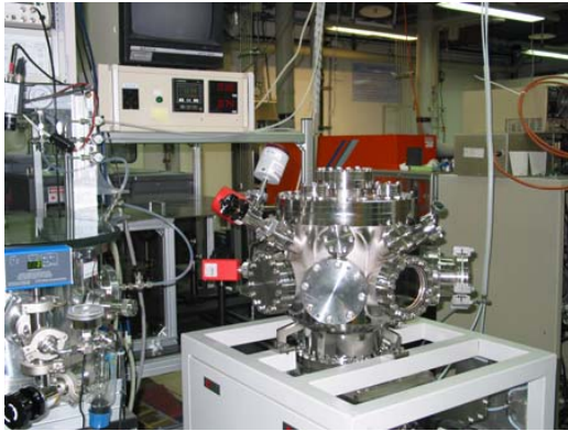
Thin film fabrication by laser ablation
