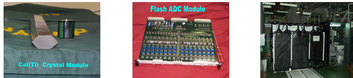
Figure 8. A 40-cm long CsI(Tl) crystal, the basic detector unit.
