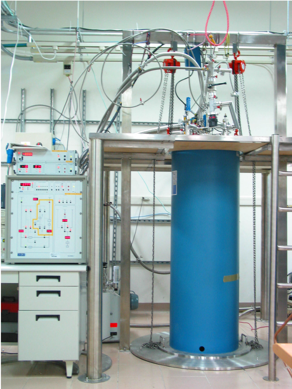
Dilution Refrigerator Kelvinox 100 Lowest temperature 10 mK and magnetic field 9 Teslas.
