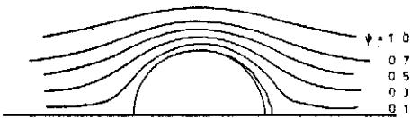
Figure 1(c) Flow Pattern at Re = 250 for T = 0.4
